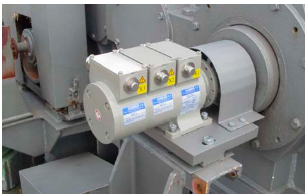
After: Electronic position switches and absolute encoder in one unit directly mounted without distribution gear.
