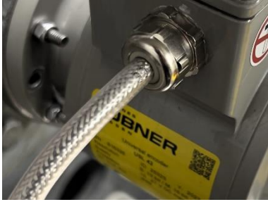
Figure 7: Original EMC cable gland on the USL(H) 42 basic unit
