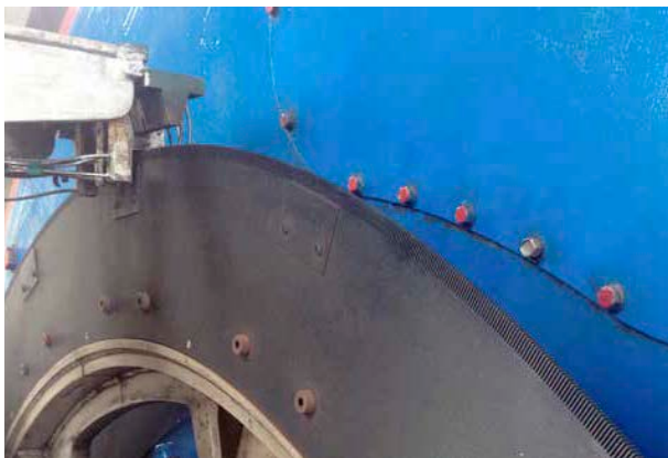
Before: The resolution of the existing optical tooth wheel scanning solution is no longer sufficient for high-precision speed control.
