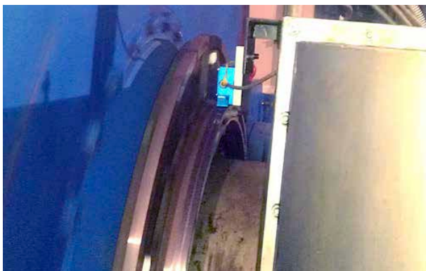
After: The tailor-made magnetic encoder system MAG 1300 provides 2460 square pulses per revolution.
