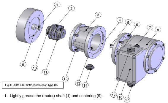
2. Fit coupling (2) onto (motor) shaft.
