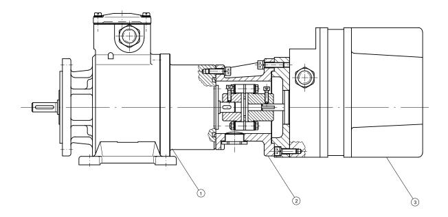
Fig.3: UOM 41L-1212 construction type B35 with coupled geared cam limit switch
