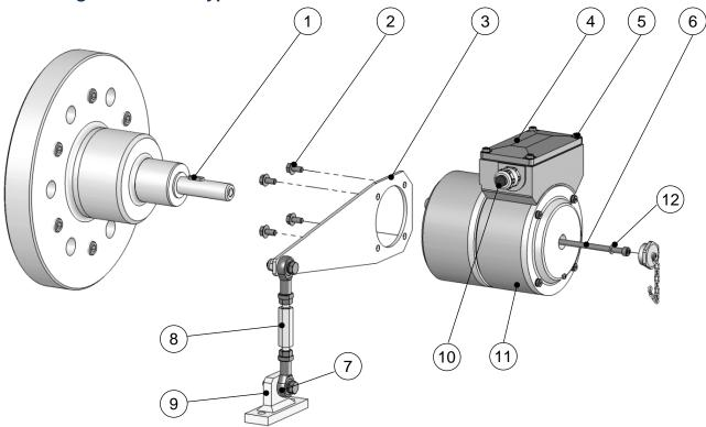
Mount adapter shaft (1) and align using dial gauge.
