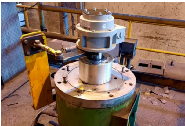
After: Hollow shaft absolute encoder type ASSH 60 K-16 / 50P with torque bracket (directly mounted)
