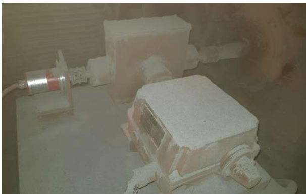
Before: Mechanical cam limit switch and absolute encoder mounted by using an additional distribution gear.
