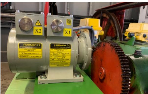
After: U-ONE-SAFETY-Compact (USC 42) with 6 safety-certified position switches (SIL 2 / PL d).
