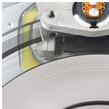
Optical scanning for high-precision signal quality and to avoid magnetic interferences
