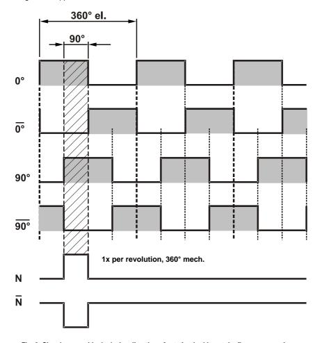
Fig. 6: Signal curve with clockwise direction of rotation looking at the flange connection
