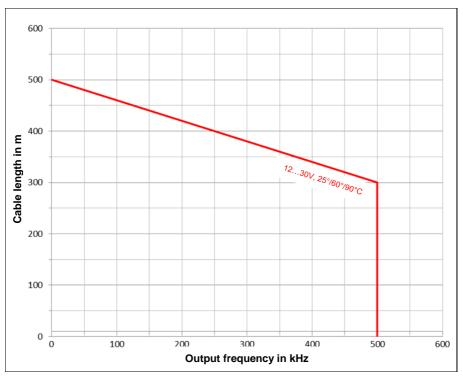
Fig. 1: Maximum permissible cable length for SIN/COS interface
