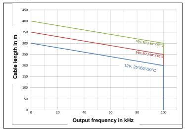
Fig. 2: Maximum permissible cable length for TTL interface
