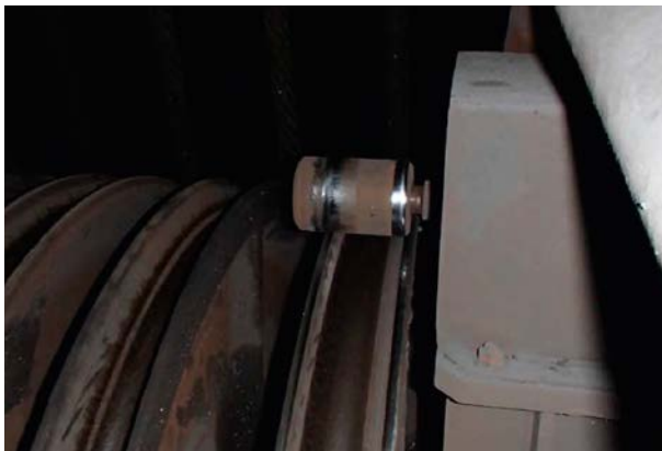
The energy for battery charging is generated from the lifting movement of the crane by a rotating sheave at the rope pulleys.
