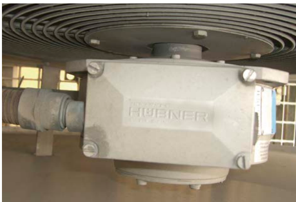
Incremental encoder FGHJ 5 with special hybrid bearings in a heavy duty housing.
