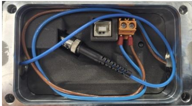
Figure: Fiber optic cable and supply cable in the terminal box of the UOM(H) 4L-1212
