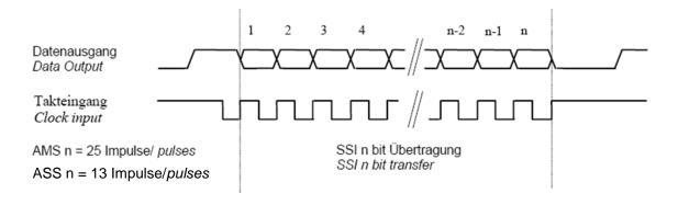
If a new data transfer is started within 20  $\mu$ s, no data reading from the code discs will be made but data of the previous cycle will be transmitted again (data repetition).
