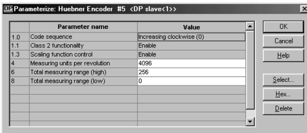
In this example, the PARAMETERIZE window shows the options for setting the parameters for an absolute encoder that has been configured for HUEBNER 2.0.
