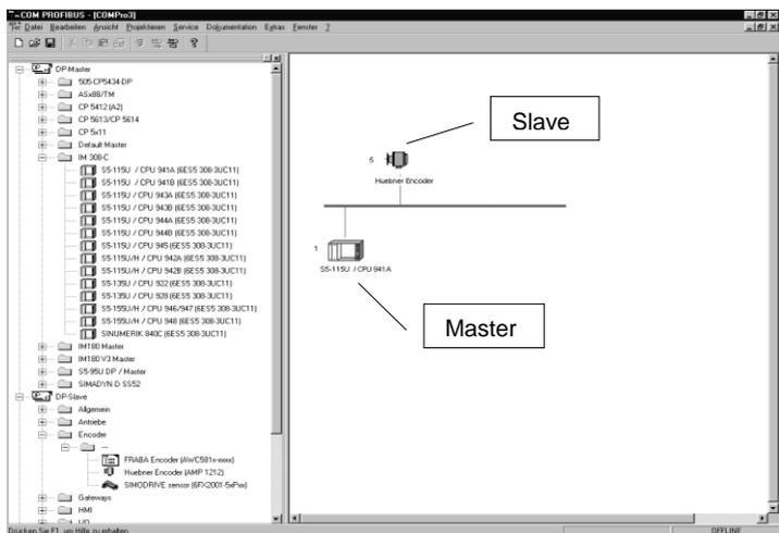
By selecting the menu item CONFIGURE / DP SLAVE CONFIGURE, or by clicking with the mouse pointer on the encoder icon, you can access the *Slave properties* window. The bus address of the encoder must be entered here, to match the setting of the address selector switches in the terminal box of the encoder.
