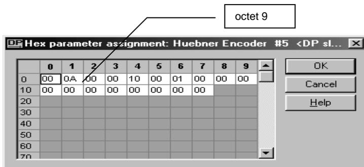
It is also possible to carry out the parameterization in the *Hex parameter assignment* window. However, this is an awkward operation, requiring precise knowledge of the functions of the individual bits and bytes.
