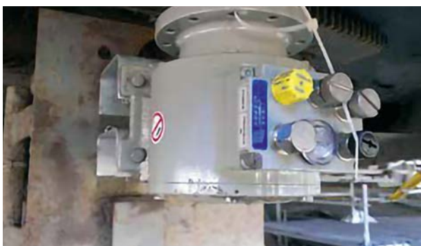
Excavadora / engranaje de giro: encoder absoluto AMPN 41 (PROFIsafe por PROFINET, SIL 3/PL d) Excavator / Slewing gear: absolute encoder AMPN 41 (PROFIsafe via PROFINET, SIL 3/PL d)
