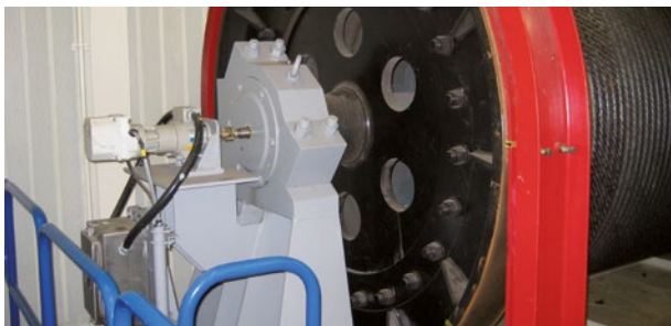
Unidade básica U-ONE® multiturn com chave de cames U-ONE® Multiturn basic unit with mechanical geared cam limit switch
