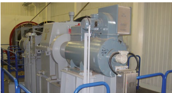
Motor equipado com encoder incremental FG(H) 40 L Motor with mounted incremental encoder FG(H) 40 L
