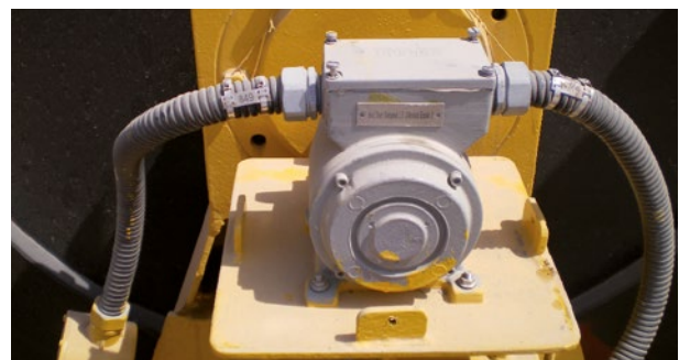
Unidade básica U-ONE® Multiturn instalada no tambor de cabos U-ONE® Multiturn basic unit installed at rope drum
