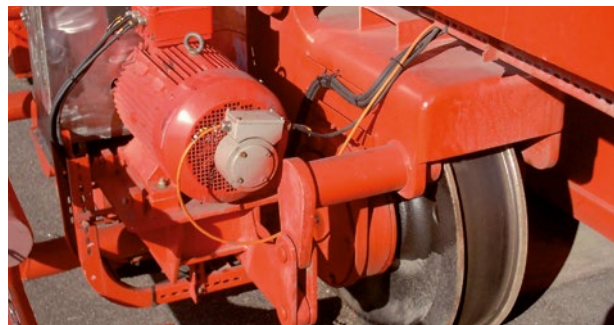
Encoder incremental FG(H) 40 L instalado no motor Incremental encoder FG(H) 40 L mounted to the motor
