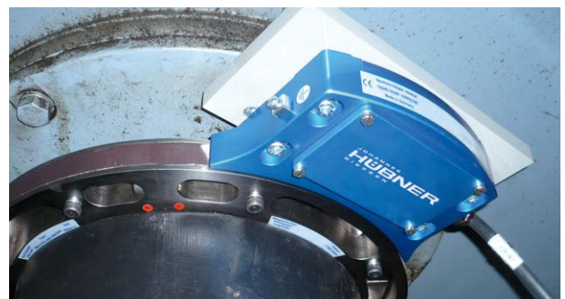
用分瓣脉冲轮实现不拆卸安装 Realization with split pulse wheel without dismantling of installation
