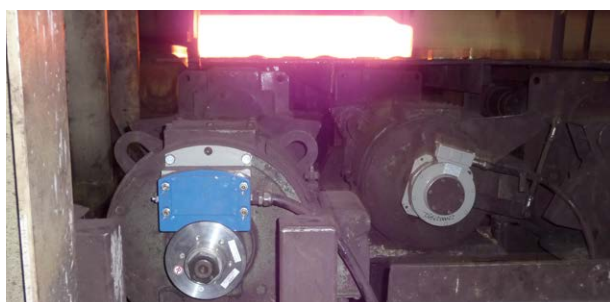
辊道电机面对高冲击和振动载荷 Roller table motors are exposed to high shock and vibration loads
