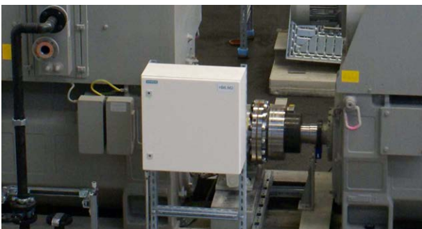
串联电机之间的连接轴上无自由轴端 No free shaft end at connection shaft between tandem motors
