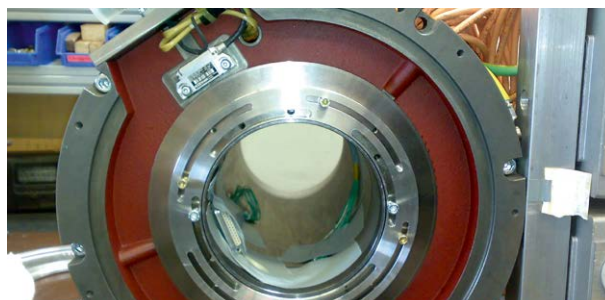
改造后：通过电机外壳直接安装定制的 MAG 系统获得精确信号 After: Precise signals through direct mounting of the customized MAG system in the motor housing
