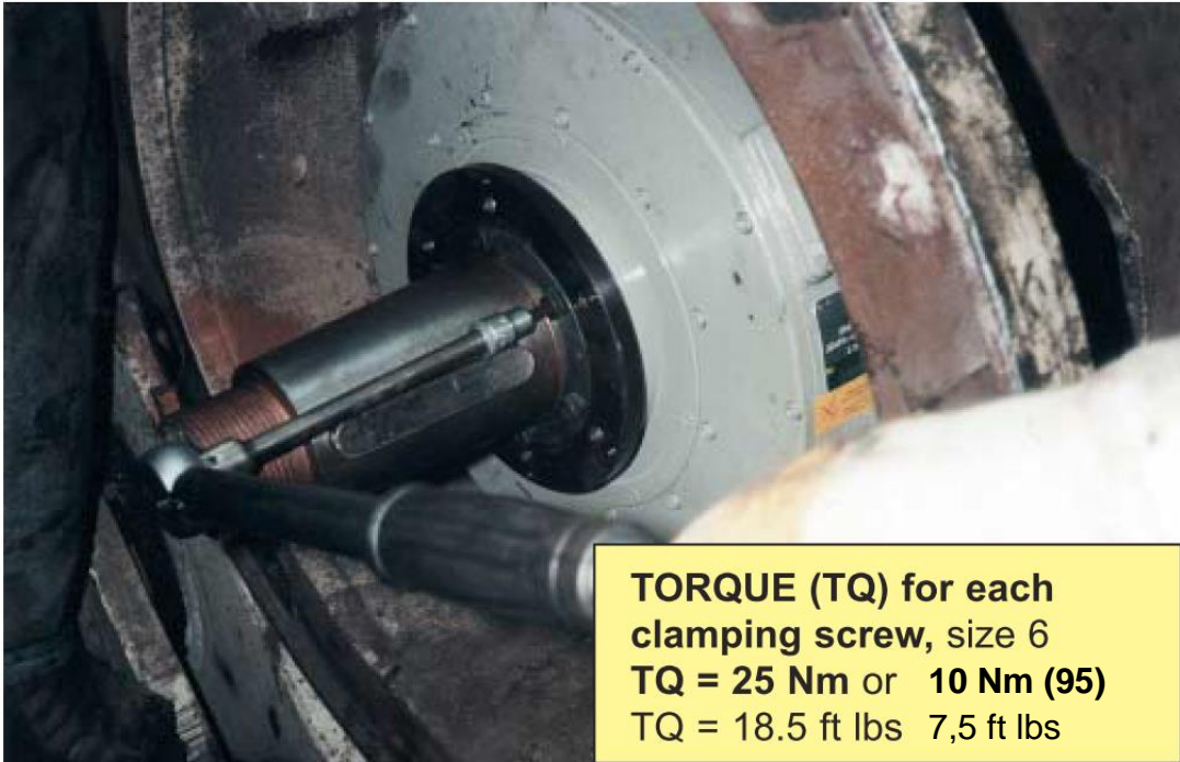
Foto shows: Spieth-Clamp of type DS 93.125.52 with hexagonal head cap screws M 8
