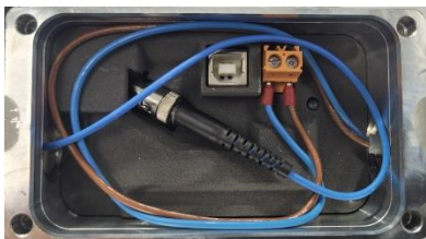
Figure: Fiber optic cable and supply cable in the terminal box of the FGH 40
