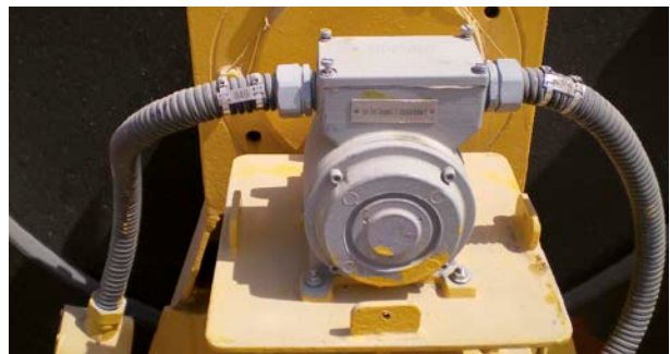
U-ONE® Multiturn Basisgerät an Seiltrommel U-ONE® Multiturn basic unit installed at rope drum
