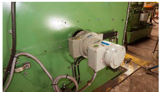
热轧 / 主传动: 空心轴绝对值编码器 ASPAH 60 (并行接口), 带电子超速开关 EGS 40 Hot rolling mill / Main drive: hollow shaft absolute encoder ASPAH 60 (parallel interface) with attached electronic overspeed switch EGS 40
