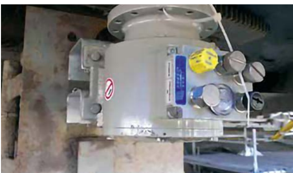
挖掘机 / 回转齿轮: 绝对值编码器 AMPN 41 (PROFIsafe via PROFINET, SIL 3 / PL d) Excavator / Slewing gear: absolute encoder AMPN 41 (PROFIsafe via PROFINET, SIL 3 / PL d)
